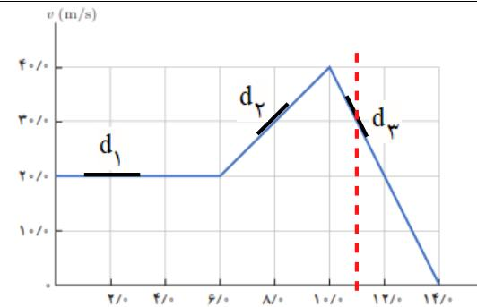
$$(الف) a_{av} = \frac{V_f - V_i}{t_f - t_i} = \frac{-20(\text{m/s})}{14\text{s}} = -1.4 \frac{\text{m}}{\text{s}^2}$$
