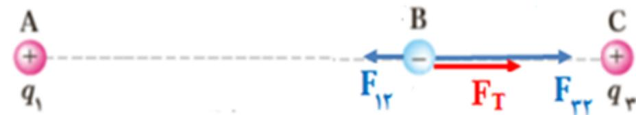
$$F_{12} = k \frac{|q_1| \cdot |q_2|}{r_{12}^2} \rightarrow F_{12} = 9 \times 10^9 \times \frac{2/\mu\text{C} \times 10^{-6} \times |-1 \mu\text{C}|}{4^2} \rightarrow \vec{F}_{12} = -1/4 \times 10^{-3} \vec{i}$$
