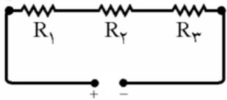
$$R_T = 12 + 12 + 12 \rightarrow R_T = 36\Omega \rightarrow I_1 = I_2 = I_3 = \frac{V}{R_T} = \frac{12}{36} = \frac{1}{3} A$$
