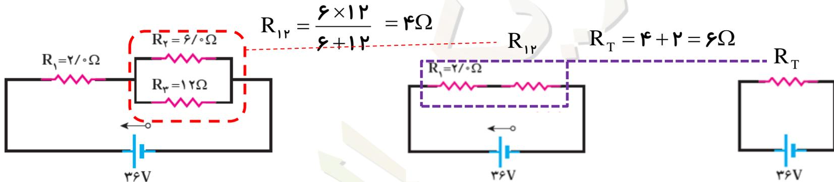
$$I_T = I_1 = I_{23} = \frac{V}{R_T} = \frac{36}{6} = 6A \quad \rightarrow \quad V_r = V_{23} = R_{23} I_{23} \quad \rightarrow \quad V_{23} = 6 \times 4 = 24V$$
